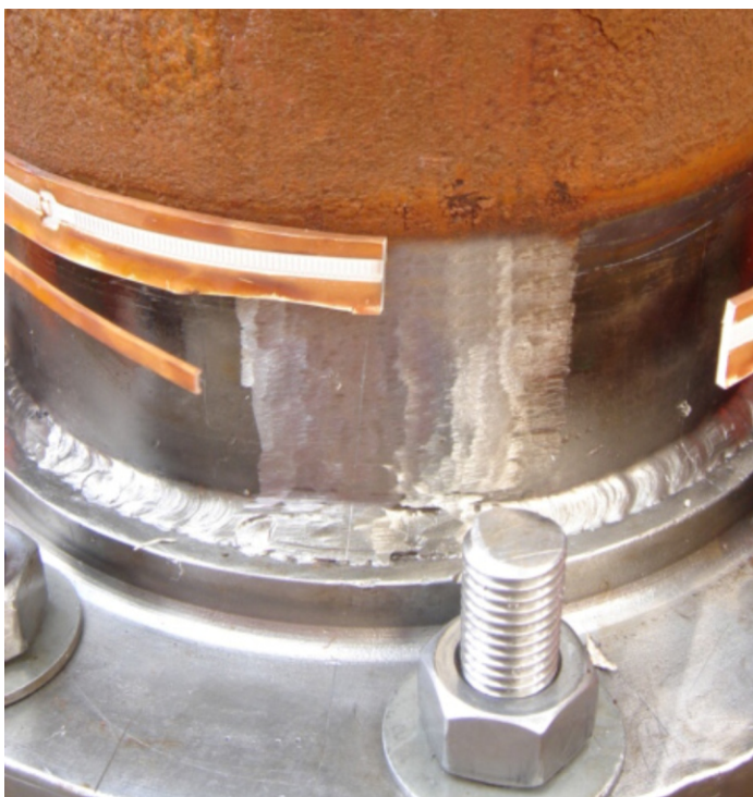
Figure 11 below: cutting through the sealing tie reveals a sharp line between the protected and unprotected areas of the substrate.
