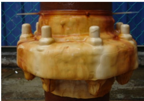
Fig 7 right: substrate after three months, just prior to removal of Enviropeel
