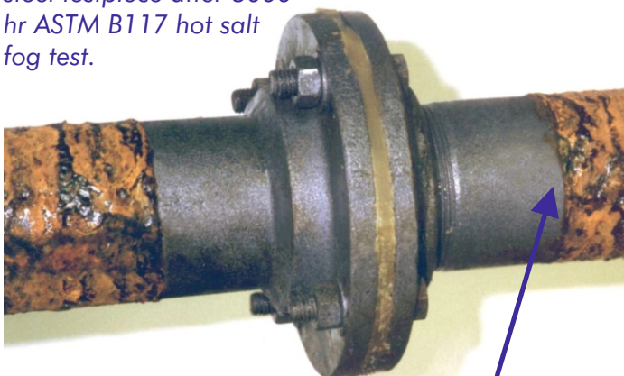
Slight 'blending' between unprotected and protected areas can be seen after removal of encapsulation.
