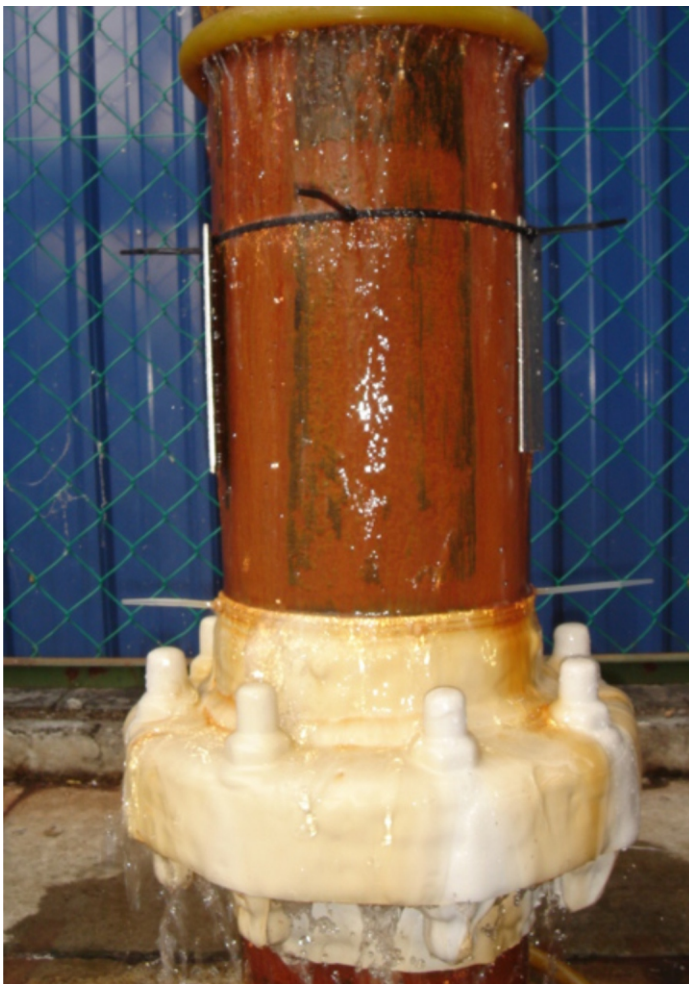
Fig 7 right: substrate after three months, just prior to removal of Enviropeel
