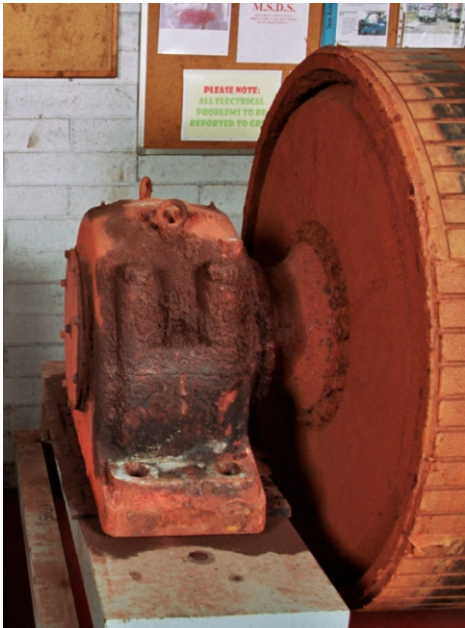
Far right: With the Enviropeel removed from a pulley housing after use, it is clear how good the performance of the Enviropeel is. The roller in the background shows clear evidence of corrosion whereas the protected pulley is as good as new.
