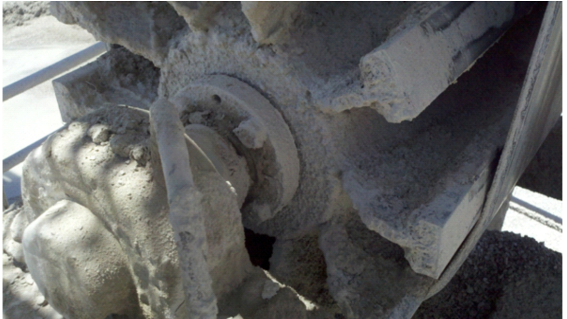
Above and below: before and after pictures show the difference between a new application and what it looks like after a year of exposure to mine conditions.
